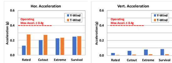
Fig. 8 Y-Wind and T-Wind nacelle accelerations
