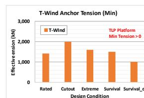
Fig. 10 T-Wind minimum tendon tension
