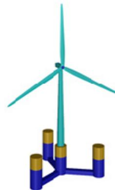
**Fig. 2** Y-Wind platform (MAS omitted)
