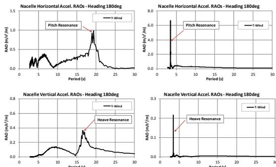
Fig. 6 Y-Wind and T-Wind acceleration RAOs
