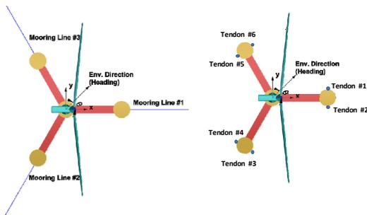
**Fig. 3** Y-Wind catenary and T-Wind tendon mooring layout
