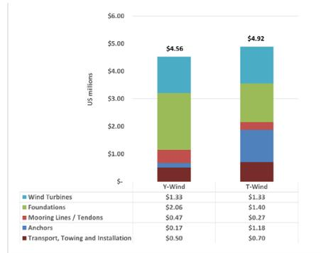
Fig. 11 CAPEX per MW by Functional Component
