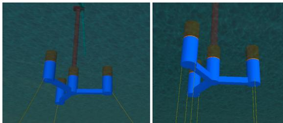
**Fig. 4** Y-Wind and T-Wind mooring layout (3-D view)
