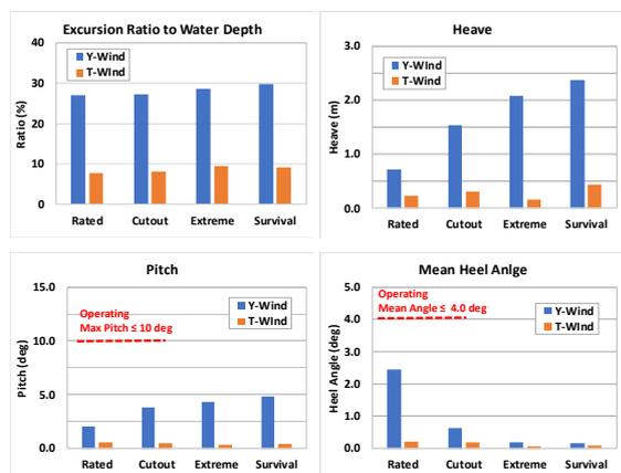
Fig. 7 Y-Wind and T-Wind motion responses
