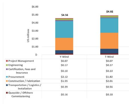
Fig. 12 CAPEX per MW by Execution Activity
