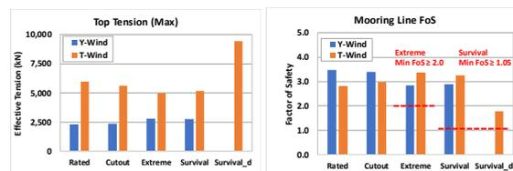
Fig. 9 Y-Wind and T-Wind mooring tensions and FoS
