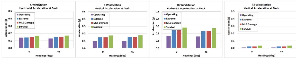
Fig. 9 Horizontal and Vertical Accelerations of X-WindStation and TX-WindStation
