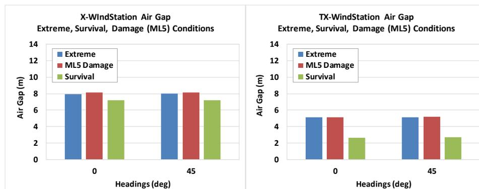
**Fig. 7 Air Gaps of X-WindStation and TX-WindStation**
