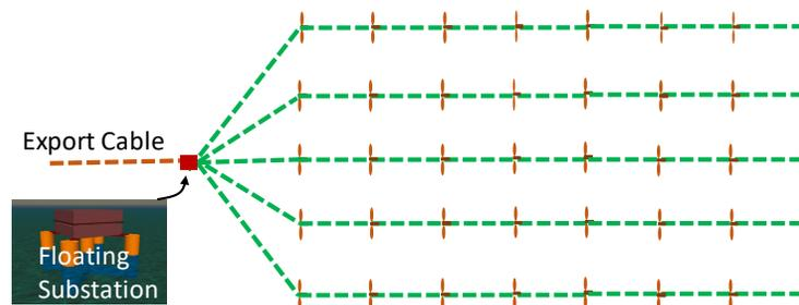
Fig. 4 Floating Substation and Typical 200 MW Wind Farm Layout with 5MW Floating Wind Platform
