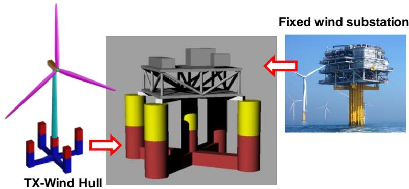
Fig. 2 X-Hull Form Floating Substation Evolutions from Floating Wind and Fixed Substation
