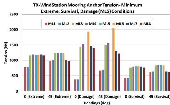
Fig. 11 Minimum Anchor Tensions of TX-WindStation
