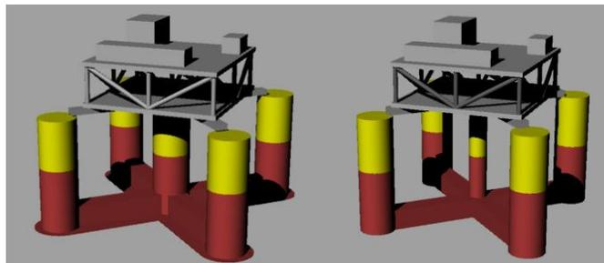
Fig 3. X-WindStation semi (left) and TX-WindStation TLP (right) type platforms
