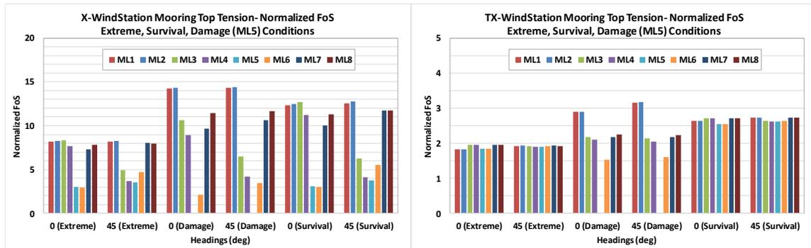
Fig. 10 Maximum Mooring Top Tension FoSs (Normalized) of X-WindStation and TX-WindStation
