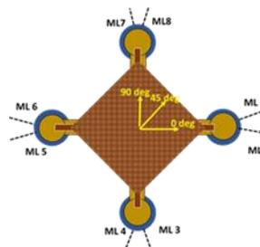
Fig. 6 Catenary Mooring Line Numbering and Heading Definition
