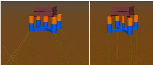
Fig. 5 Mooring Layouts of X-WindStation (left) and TX-WindStation (right) from Numerical Model
