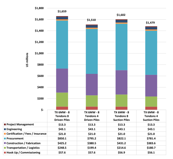
Fig. 15 CAPEX of wind farm by execution activity: 34 units of 6 MW TX-Wind
