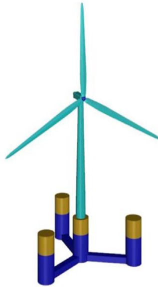
Figure 5—Y-Wind Semi with HAWT Turbine on Center Column
