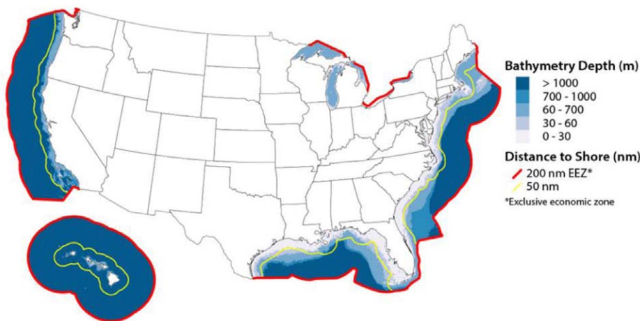
Figure 2—Gross Potential Resource Area Showing Excluded Water Depths of More than 1,000m in Dark Blue (Musial et. al, 2016, Fig. ES-1)
